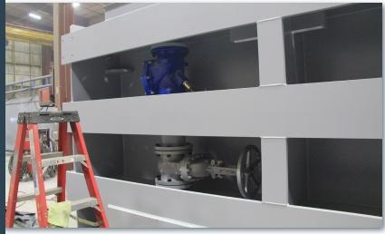
Onaway, MI - MIW has completed and delivered (4) sets of Upper and Lower stop logs to the Rock Island Dam in Rock Island, WA. The project was devised from a need to update the current stop log system in place at the Rock Island Dam. The project primarily consisted of A572-GR 50, a high strength, low alloy steel and A276 304 Stainless Steel, a product that offers good corrosion resistance.
