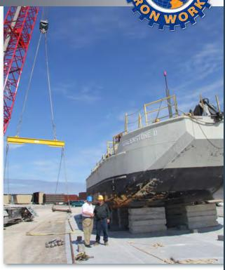
The GREENSTONE II, a U.S. Department of Interior fuel barge, was hauled out at the Port Calcite facility in late May 2014 with MIW's 440-ton Manitowoc 16000 crane. Schwartz Boiler of Cheboygan, MI performed the blasting, painting, and repair work. Upon completion of drydocking, repair work, and inspections by the U.S. Coast Guard, the barge was relaunched at Port Calcite in late June.
